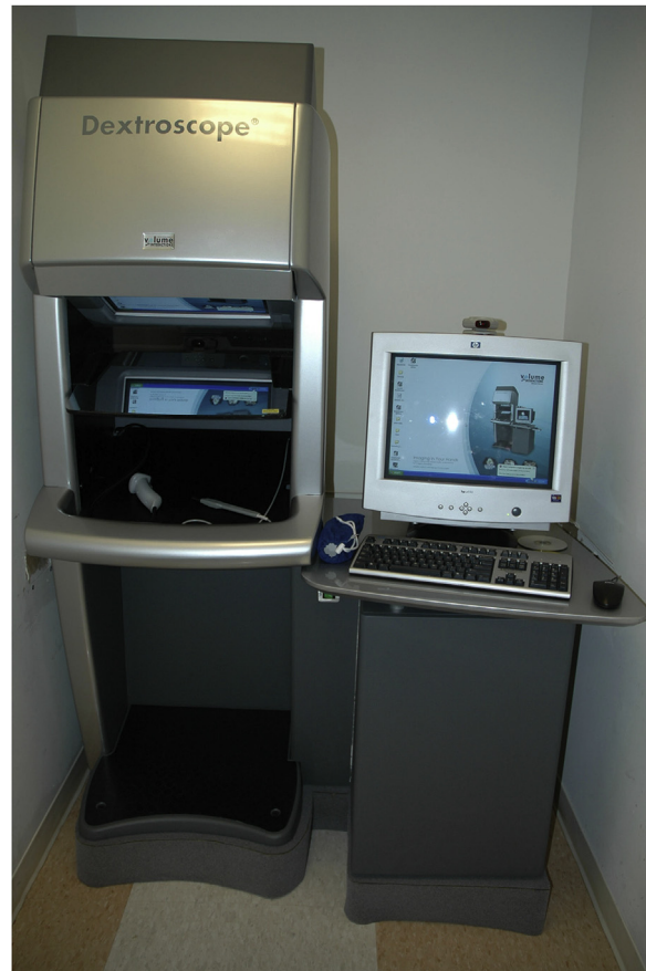
Fig. 1. Image of the Dextroscope® virtual reality system, by Volume Interactions. The left-hand side shows the interface for virtual reality users, including a handle (“joystick”). The right-hand side shows the interface for experimenter or teacher.
